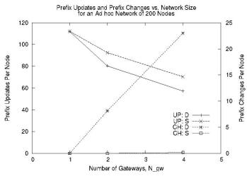
Figure 6: Number of prefix updates (left axis) and prefix changes (right axis) versus the number of mobile gateways.
