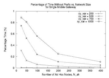
Figure 5: Percentage of time without a prefix per node plotted against various node densities.
