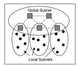
Figure 1: The logical network topology under consideration. Leaders, denoted by squares, form the backbone and serve as attachment points for the subordinates, represented as dots.
